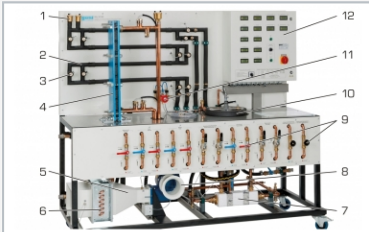
1 bleed valve, 2 tubular heat exchanger, 3 temperature sensor, 4 plate heat exchanger, 5 air duct, 6 finned tube heat exchanger, 7 shell & tube heat exchanger, 8 fan, 9 adjustable fittings, 10 stirred tank with double jacket and coiled tube, 11 pressure sensor (water), 12 switch cabinet
